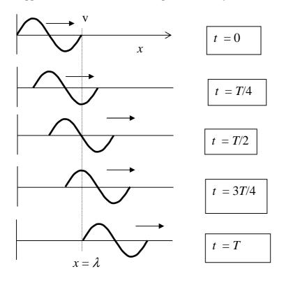
The length of one full cycle of the wave is called the wavelength  $\lambda$  m. Travelling at velocity v it takes a time T s given by
