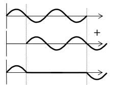
Two waves Out of phase  $\phi = \pi$  radians
