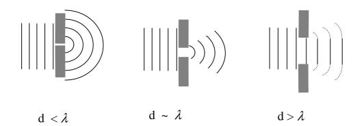
Diffraction of plane waves by a pinhole (or slit). The diagrams attempt to depict something that is more complex in practice. Just like any other wave motion light is subject to diffraction and its influence can limit the focus of instruments – such as the **pinhole camera**
