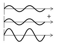
Two waves in phase (coherent):  $\phi = 0$ .
