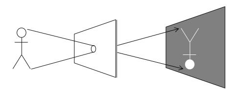
Blurring of the image happens because rays from the head (say) can pass either through the top of the hole or the bottom (this is geometric optics). Thus, the smaller the hole the better (if dimmer) the image. But if the hole is *too* small the wave properties of light become important and the image is blurred by diffraction effects.
