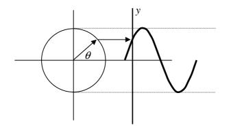
The height  $y = A\sin(\theta)$  if A is the radius of the circle. The angle  $\theta$  is called the *phase* angle and can be used as a measure of position along the waveform. In this measure the
