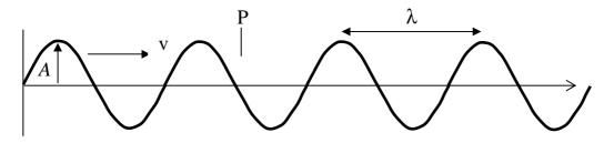
Here the distance between crests is the easiest way of measuring the wavelength. The number of crests that pass an arbitrary point P in one second is termed the *frequency*, f, and is usually expressed in Hertz (Hz), or cycles/second. If one crest passes point P in time T seconds, then the number of crests passing in one second is the frequency f
